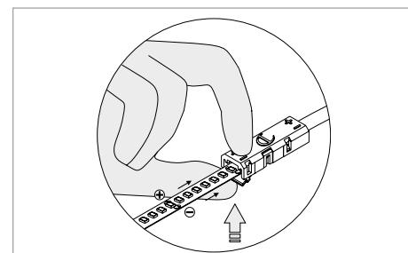
It is recommended not to bend the light sources during handling and assembly as this could impair operation. Refer to the assembly instructions supplied with the product for more details.
