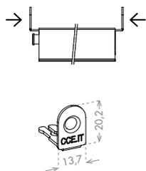
This symbol indicates that the automatic drop-down seal can be fixed with lateral steel brackets. All the versions available for each product are specified in the image.
