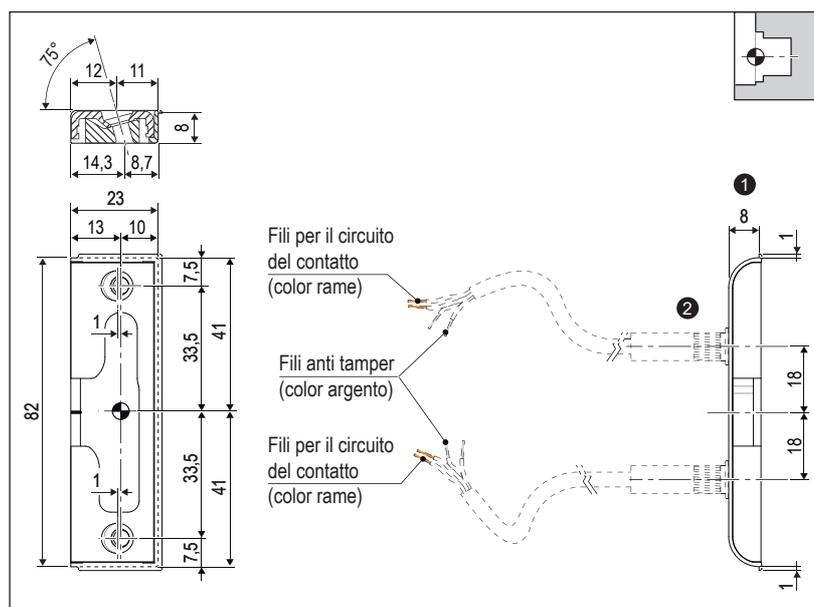
**Aria 4 mm, interasse 13 mm, viti inclinate**
