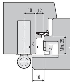
**FRESATE PARTE TELAIO**
